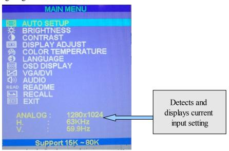
**Please Note:** Due to the advanced nature of this panel. Adjustments to clock, phase and image positioning are saved only for the signal timing you are currently using. Meaning if your input is CGA 640 x 215 @60Hz, and you adjust the clock setting. This will only affect this timing.
