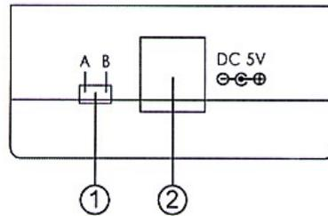
1. Input Selection: Use this mini switch to select from 2 input ports A and B.
