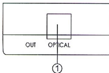
1. TOSLink (Optical Fiber) Output Port: Connect the TOSLink output port to the TOSLink input port of audio equipment such as audio amplifier and AV receiver.
