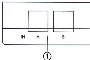
1. TOSLink (Optical Fiber) Input Ports A and B: Connect the TOSLink input ports to the TOSLink output port of audio equipments such as audio amplifier, AV receiver or DVD player.
