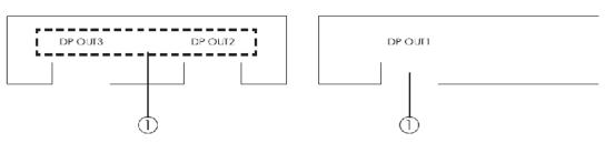
① **DP OUT 1~3:** Connect these slots with the output displays Display port input port in order to send a signal.
