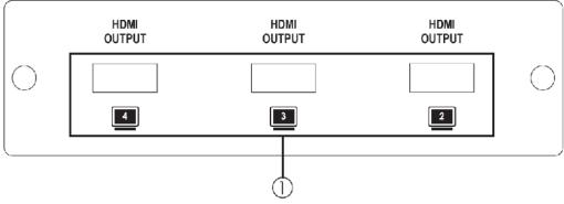
① HDMI Outputs 2/3/4: Connect each of the output ports to the HDMI display. When more than one output connected, the HDMI outputs play identical video signal simultaneously.
