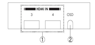
(1). HDMI IN 3 & 4: These slots are where you connect the input source devices for sending a signal to the input source with HDMI cables.
