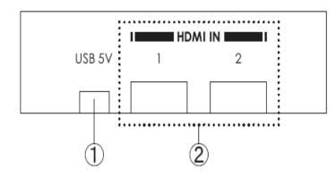
(1). **USB 5V:** This slot is where you can connect the mini USB cable from your PC to the device in order to supply power.
