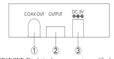
①. COAX OUT: This slot is where you connect an amplifier for transmitting an audio signal with coaxial cables. When the audio return function is on the audio signal will be received from the output and when the audio return function is off the audio signal will be received from the input source.
