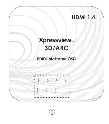
1. Input LED 1~4: These LED will switch on according to user's input selection.
