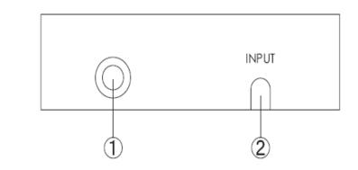
(1). **IR sensor: T**his is a IR receiver window that receives IR signals from the remote control included in the package.
