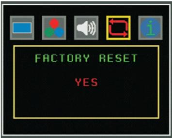
• Select YES to return to the factory setting. Factory setting on display is at 1024 x 768@60Hz with full size screen, Color setting's factory default rate are as the value in the bracket of the OSD chart and SDI audio is on auto.
