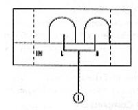
**1.** L/R input: Connect L/R stereo analog audio input port to the L/R source equipment, such as DVD player or PS3.
